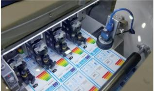
The cutting module with double cutter heads ensures the cutting speed and optimizes the operation steps. The enclosed cutting module greatly improves the safety of operation.
