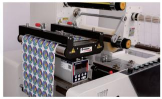
The width of feeding and die cutting reaches 320 mm which can meet the needs of most label manufacturers. Equipped with a guided deviation correction system, the feeding is more stable.
